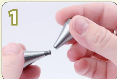
1 Screw both sides of the Hourglass Mandrel together.
