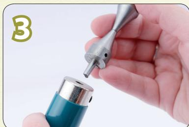
3 Insert the Hourglass Mandrel into the Conetastic Tool (sold separately) with the flat side of the mandrel shank aligned with the set screw.
