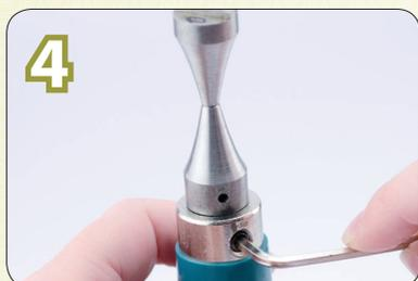
4 Use an Allen Wrench to tighten the Hourglass Mandrel into place.
